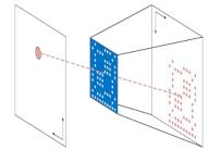
Left: Coded Aperture in comparison to other collimation techniques. Right: The lateral position is encoded by the shadow's shift, the axial position by the shadow's size.
